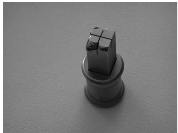
Fig. 1. Sample 1 after exposure in the FTU scrape-off layer (the sample is shown inserted in the sample carrier).
